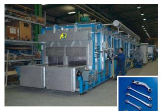
Heating of cast automotive suspension parts for a downstream forging operation (COBAPRESS® process), loading side 2.5 t throughput, open natural-gas heating
