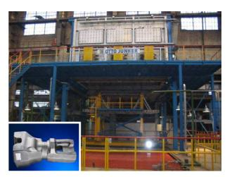
Examples: Drop-bottom furnace systems for solution annealing large forgings for the aircraft industry. Direct electric heating, stationary water quench in a pit, charging car serving as load and unload station and for charging the furnace.
