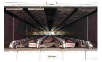
Interior view of the solution annealing furnace; two tracks; all-internal chain conveyor  $% \left( {{\left[ {{{\rm{ch}}} \right]}_{\rm{ch}}} \right)$
