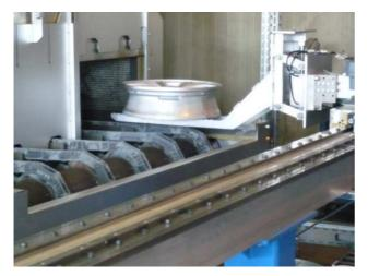
Loading operation by means of a manipulator
