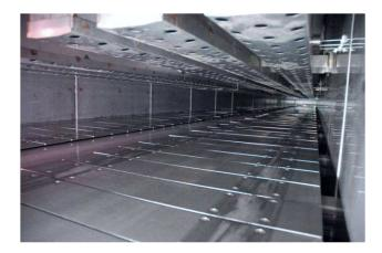
Interior view of the furnace with jet heating nozzle beams, dual-track conveyor, independent track control
