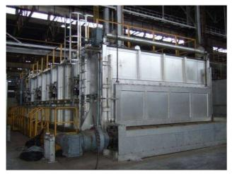
Pre-heating furnace for forgings, 8 t/h throughput, open natural-gas heating
