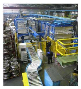
Heat treatment system for forged aluminium wheels, directly linked to the flow forming process
