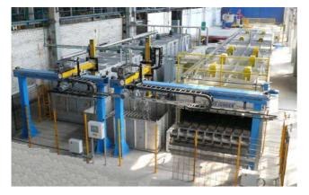
Heat treatment systems for forged aluminium wheels, consisting of the solution annealing furnace (2 tracks), water quench, artificial ageing furnace (4 tracks), loading and unloading manipulators
