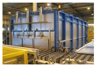
Wheel heating furnace before flow forging
