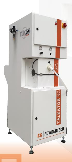
The powdering is done by 1-2 **AST** powder guns connected to up to two jet pumps. The new, patented coating technology **RS AirStreamTechnology**<sup>®</sup> is able to achieve a very fine and even coating on the product at production speeds of up to 100 m/min, even without electrostatics.
